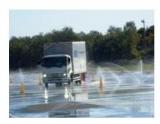
Actually experiencing slippery road surfaces on the low friction test course
