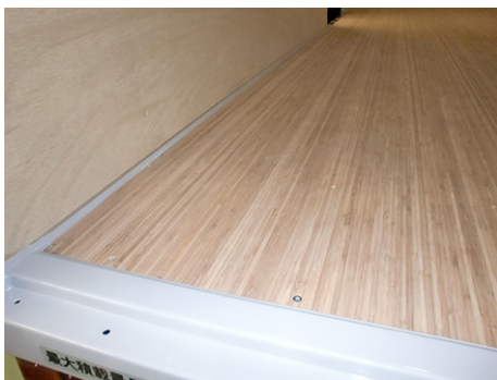
A vehicle utilizing bamboo flooring material
