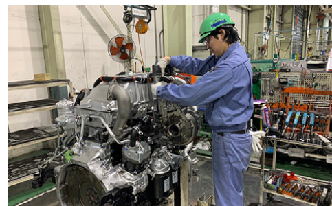
Rebuilt Engine Reassembly
