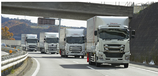
Highway validation test for truck platooning
