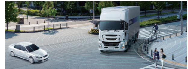
Blind spot monitor that projects from the cab in four directions
