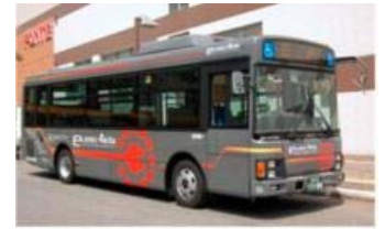
In Akita City runs the Elemo-Akita, an original bus based on the Isuzu ERGA Mio.
