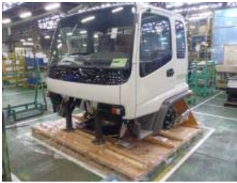
Packaging cabs and axle cases into one case. The cabs and axle cases were previously individually packaged.
