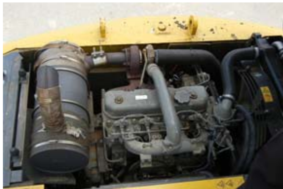
Restored Engine Mounted
