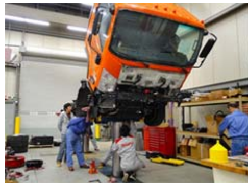
Disassembled analysis on water-damaged vehicle
