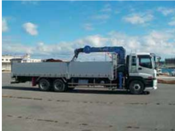
Truck with a crane mounted directly behind the cab, imperative for fixed net fishing
