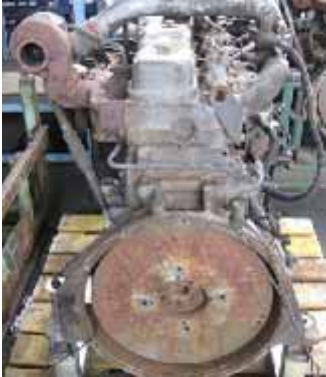
Rusted engine after water damage
