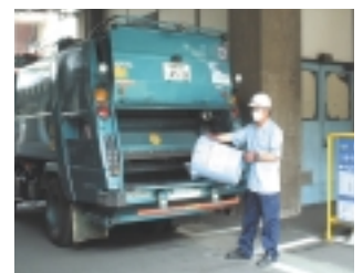
Waste collection by garbage compressor truck, similar to the type used for household garbage.
