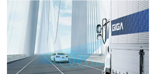
Pre-crash brake control that can detect pedestrians and bicycles
