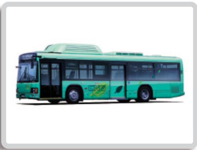
Isuzu has developed a CNG (compressed natural gas) vehicle for use as a non-step large route bus. The vehicle boasts extremely low levels of harmful exhaust emissions. Some models also employ an oxygen catalytic converter to reduce levels of particulate matter. These innovations mean the vehicle has an exceptionally low impact on the environment. (Domestic model)
