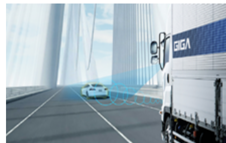
Pre-crash brake control that can also detect pedestrians and bicycles
