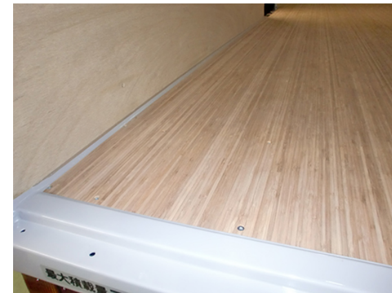
A vehicle utilizing bamboo flooring material
