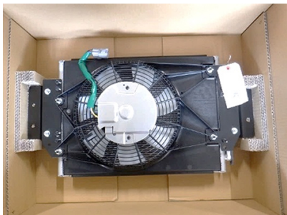
Packaging of parts using corrugated cardboard fixing material
