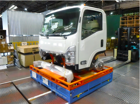
Cab returnable rack (orange) + parts returnable rack (blue)
