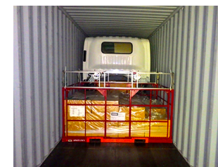
Inside and outside of the container for shipping KD parts in the CRU system
