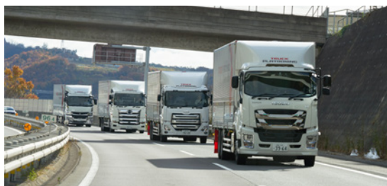
Highway validation test for truck platooning
