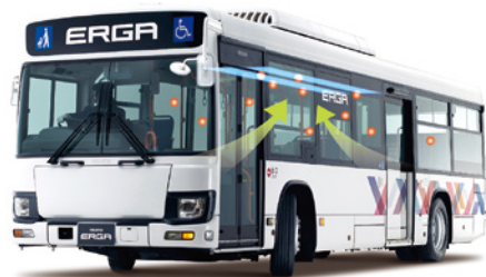
Image of droplet nuclei being captured by an aerosol filter
