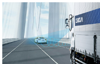
Pre-crash brake control that can detect pedestrians and bicycles
