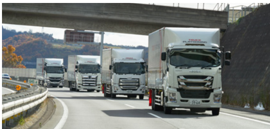
Highway validation test for truck platooning
