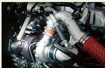
**Electrically controlled continuously variable geometry turbochargers**
