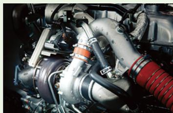
**Electrically controlled continuously variable geometry turbochargers**
