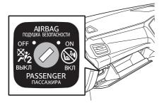
The passenger side SRS airbag on-off switch is positioned below the instrument panel on the passenger side. Open the glove compartment to check the switch. Always ensure that the passenger side SRS airbag on-off switch is in the proper position before driving.
