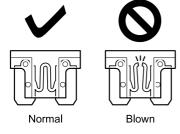
If the fuse appears is as shown in the right-hand side of the diagram at left, the fuse is blown. Replace with a spare fuse. Spare fuses are stored in the fuse box inside the engine compartment and within the instrument panel.
