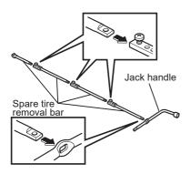
1. Assemble the spare tire removal bars and jack handle.
