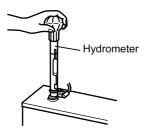
Check the specific gravity of the battery fluid using a hydrometer. If the specific gravity is too low, the battery should be charged.
