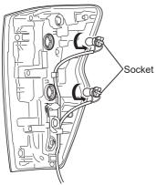
2. Turn the socket of the replacing bulb counterclockwise to remove it.
