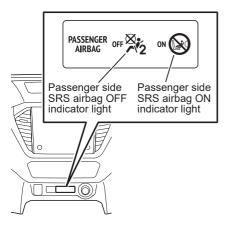
Passenger side SRS airbag ON indicator light
