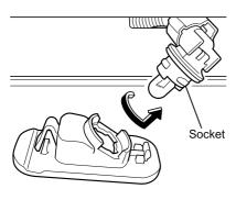
3. Loosen the socket by turning it counterclockwise.
