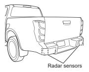
Radar sensors are installed on the inner right and inner left sides of the rear bumper.
