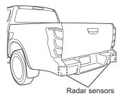
Radar sensors are installed on the inner right and inner left sides of the rear bumper.
