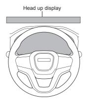
The head up display projects LED light onto the windshield to alert the driver.
