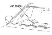
The air conditioning system uses a sun sensor, interior temperature sensor and outside air temperature sensor to ensure effective and comfortable air conditioning. Do not place anything on the sensors or get them wet. Air conditioning control will become inaccurate.
