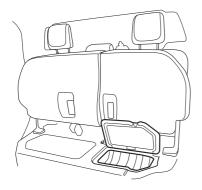
The storage compartment is under the rear seat.
