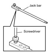
When assemble jack bars to each other, tighten joint bolt by hand or a screwdriver (Phillips side).
