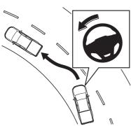
The system recognizes lanes and assists the steering wheel operations to keep the vehicle driving in the center area of the lane while the adaptive cruise control is set. The system operates while the vehicle speed is below 130 km/h (80 MPH) (automatic transmission models) or from 30 to 130 km/h (19 to 80 MPH) (manual transmission models).
