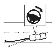
When the vehicle is about to depart from the lane while the LDW is issuing a warning, the system assists the steering wheel operation in the direction to avoid lane departure to control departure from the lane.
