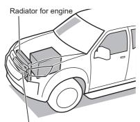
Radiator for water-cooled intercooler
