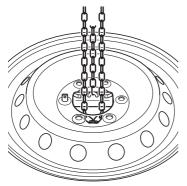
Let the chain rest in the center of the disc wheel while it is raised halfway. Then turn the jack handle to lift up the tire.
