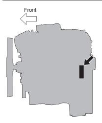
The engine number is stamped on the left side rear part of the engine block.
