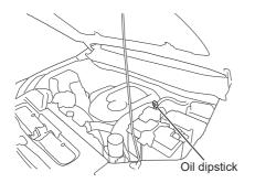
Perform the engine oil level check on a flat surface while the engine is cold before starting it. If the engine has already been started, stop it after it has sufficiently warmed and wait 30 minutes or more before performing. Also, check if there are any oil leaks and
