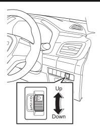
The headlight aim can be adjusted at four different angles. When the cargo load causes the headlights to aim upwards, this feature can be used to lower the aiming angle.
