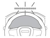
The forward collision warning (FCW) light is a warning light that flashes just before the automatic brake is activated to alert the driver to a risk of a collision with a pedestrian, cyclist, motorcyclist, vehicle, or obstacle in the forward direction.
