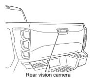
The rear vision camera is installed to the tailgate.
