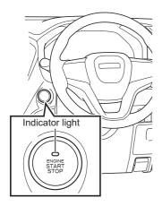
This button is used to start/stop the engine and switch the power mode.
