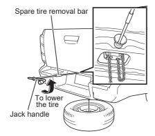
Insert the spare tire removal bar into the hole in the spare tire carrier, and turn the jack handle counterclockwise.
