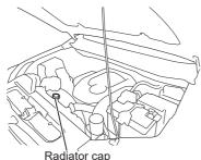
The reserve tank is located at the front right side of the engine compartment. When the engine has cooled down, make sure that the engine coolant level in the reserve tank is between the "MAX" and "MIN" line. In addition, remove the radiator cap and check that the engine coolant is full to the filler neck. Check the engine coolant level only when it is cold.
