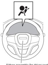
Airbag assembly for driver seat
