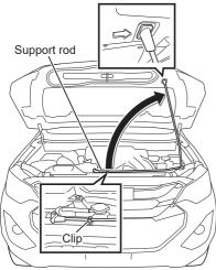
Remove the support rod from the clip, and then install the support rod edge hook into the groove of the engine hood.
