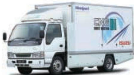
Isuzu exhibited the prototype direct-injection, diesel-cycle, mono-fuel, CNG-powered ELF light-duty truck in collaboration with Westport Innovations, Inc. of Canada at the Michelin Challenge Bibendum, considered one of the premier global events for advanced technology vehicles.
