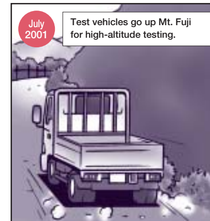
10 Another challenging issue was to demonstrate engine performance at high temperatures. The engine must be tuned so that coolant water temperature does not rise too far, reducing engine power, even when the gas pedal is floored while the truck is climbing a steep slope.
