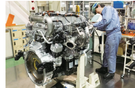
Rebuilt engine in the midst of being reassembled
